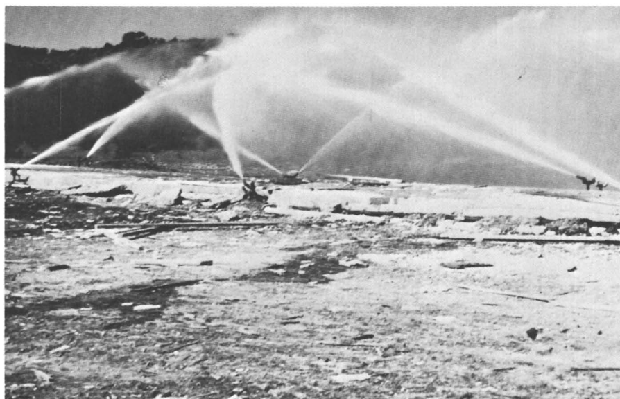
Figure 25. Operating nozzle system following detonation of donor box
