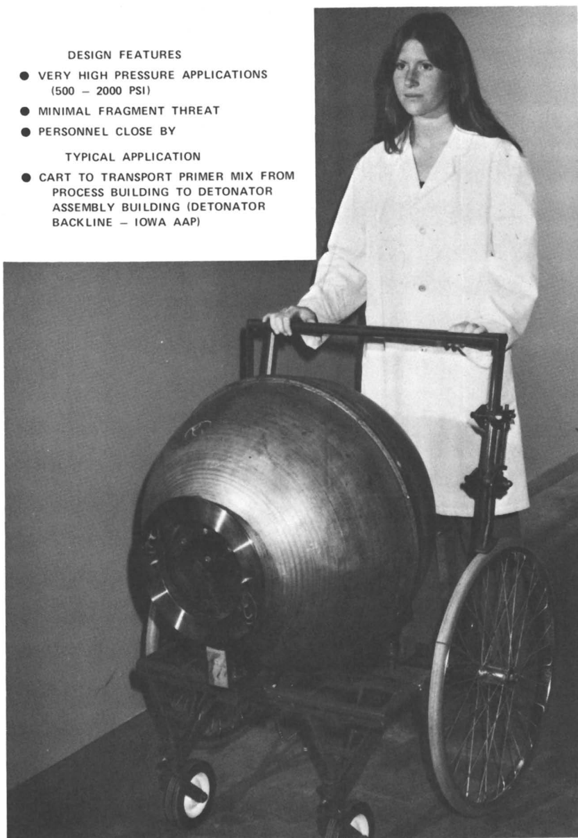
Figure 5. Group 6 suppressive shield cart
