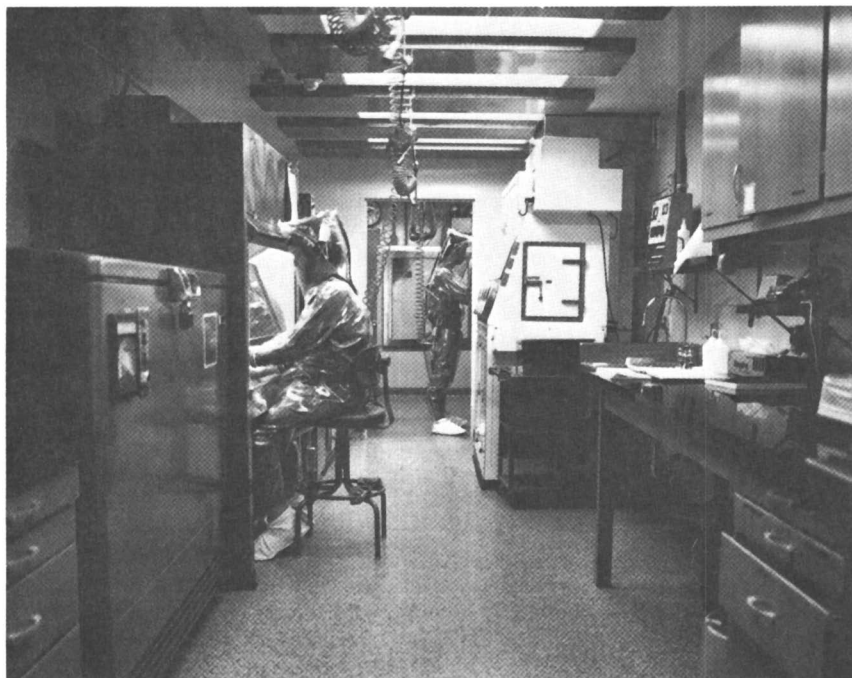
Figure 2. Respiratory protective equipment. One-piece positive pressure ventilated suits. Mine Safety Appliances Company
