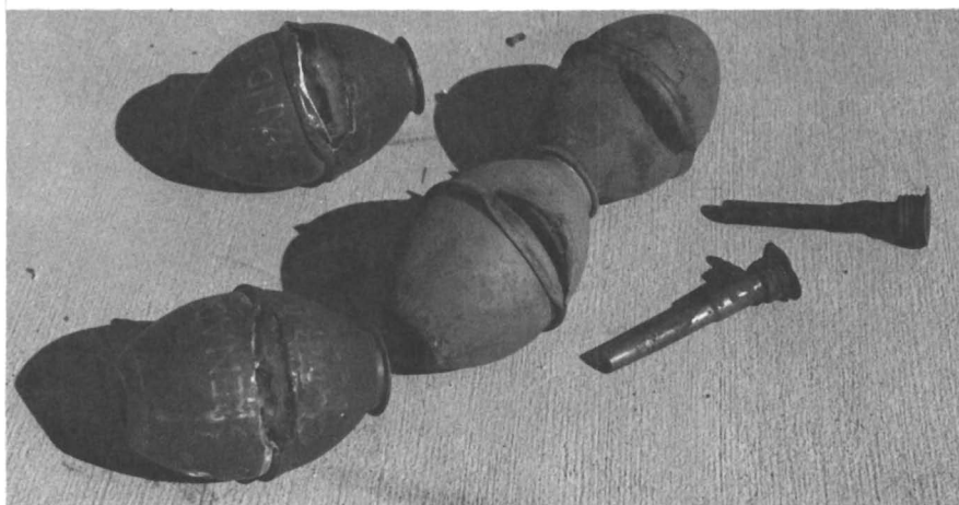
Figure 2. M26 grenades, sheared and burned
