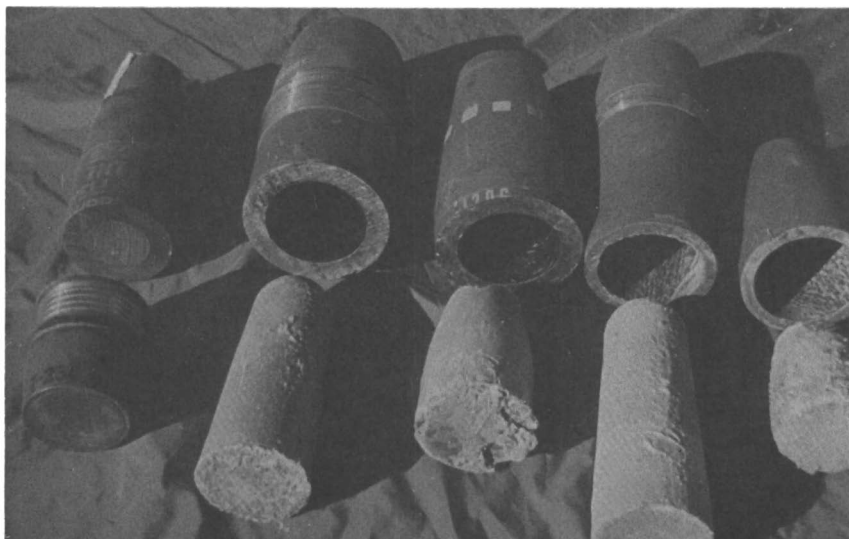
Figure 5. TNT and composition B severed projectiles before and after melt out
