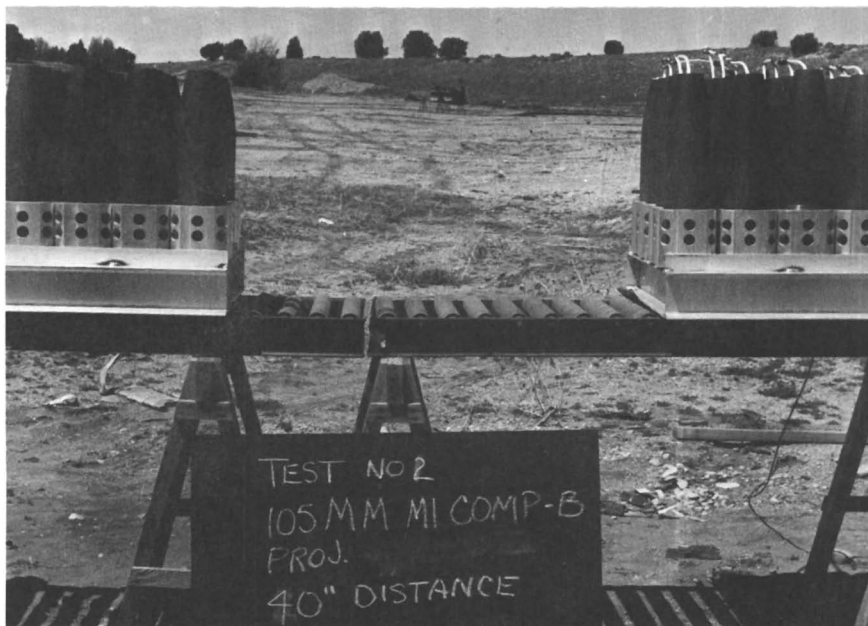
Figure 10. Test arrangement with 16 projectiles primed
