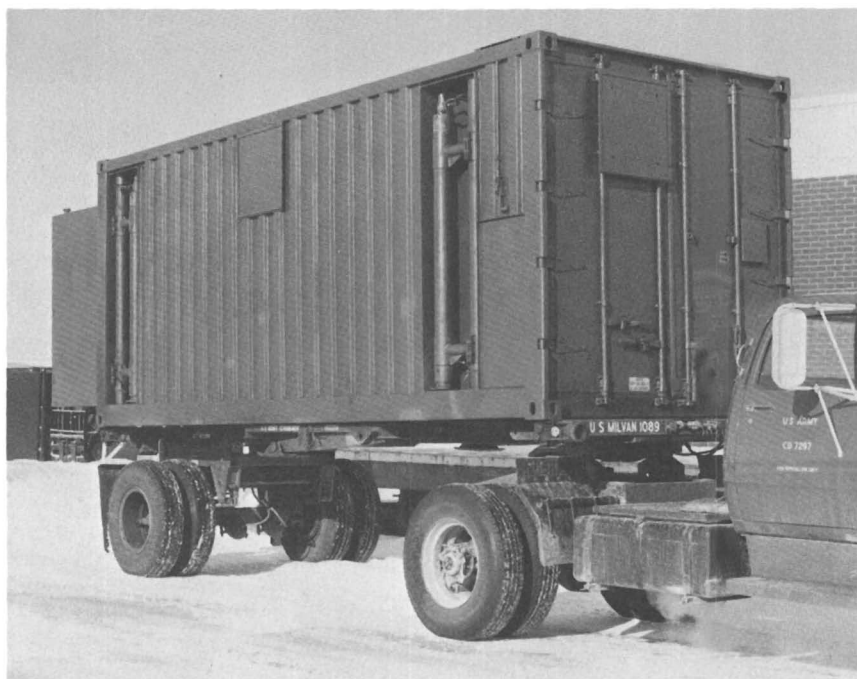
Figure 9. Mobile Surveillance Inspection Shop mounted on MILVAN chassis ready for movement
